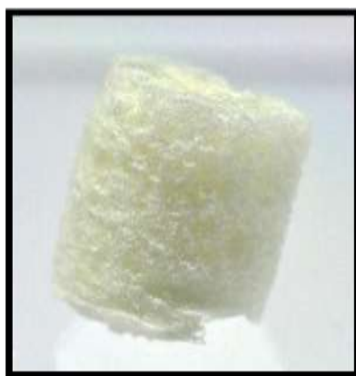
Figure 2. Porous scaffold composite with highly porous and opening pore structure
