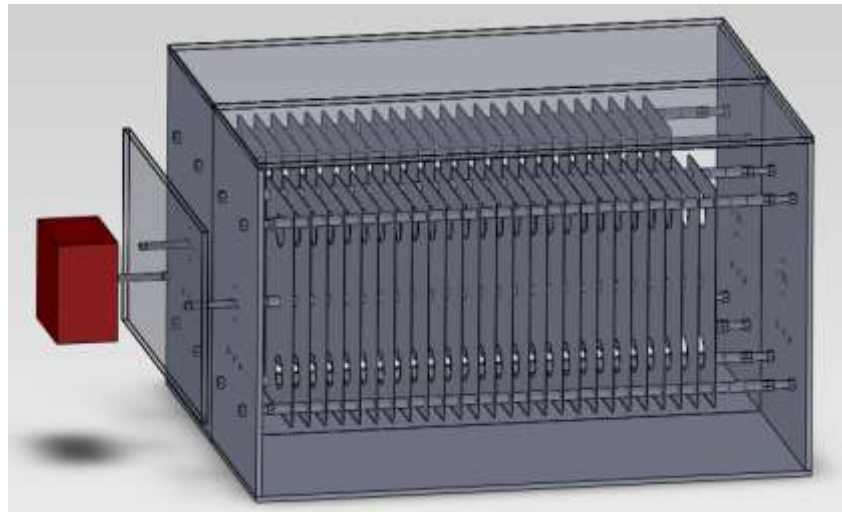
Fig. 3(c). Parallel connection and one exciter with a connecting plate
