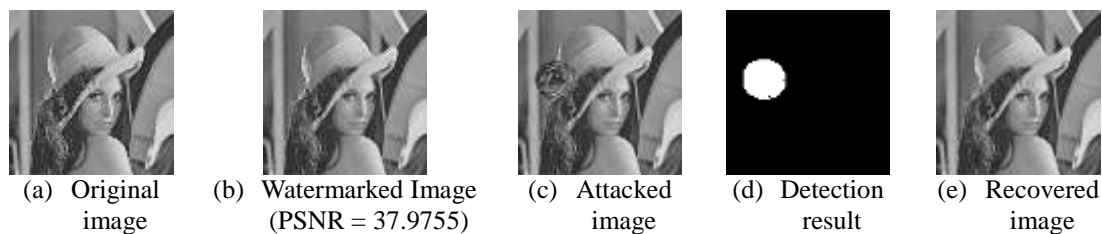
Figure 2 The original and watermarked images of the proposed scheme
