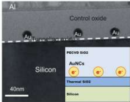
Fig. 1. The cross-sectional TEM picture and diagram of device structure.
