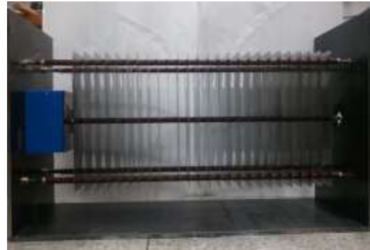
Fig. 1(b). The Prototype of single ESP system
