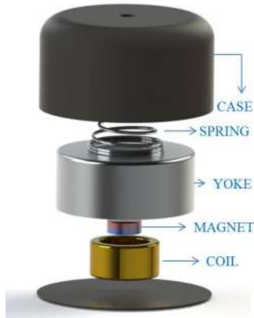
Fig. 1 Schematic diagram of typical horizontal linear vibrating actuator
