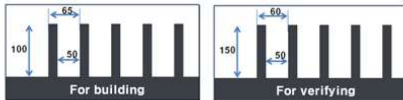
Fig. 5: The rectangular pattern's shapes for building (left) and verifying (right)
